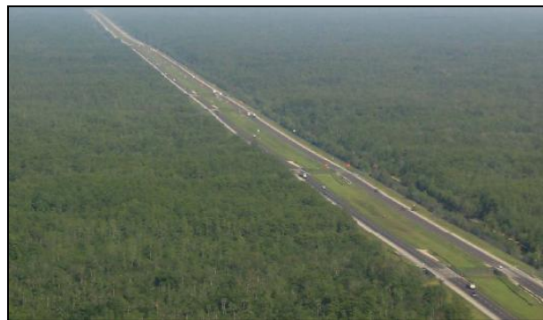
Image 5.1: The 64 km I-75 project area has 36 underpasses across 4 lanes of divided highway. Source: Lotz & Land, 2007.
